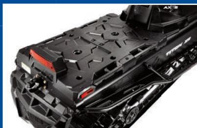
**LOCK & RIDE® PLATFORM** Integrated design allows for maximum storage, with or without passenger seat. A huge 85lb. (38.5 kg.) carrying capacity and integrated Lock & Ride mounting system holds cargo box and other storage accessories.
