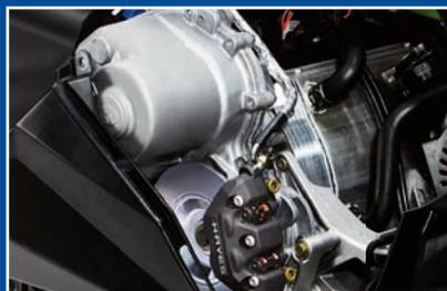
**ALPHA TRANSMISSION** Provides smooth shifting and drive ranges to suit even the most extreme conditions or situations. 1200 lb. towing capabilities with High, Low, Reverse, and Neutral.
