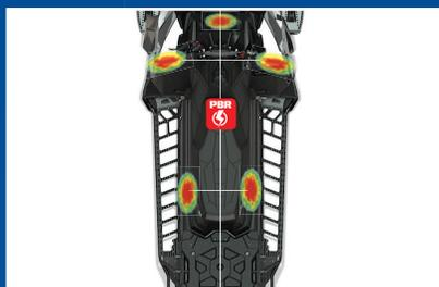
**POWER BOOSTING REGULATOR** This patented industry-first delivers maximum electrical power at idle and low RPMs. Ensures power for rider comfort and convenience features, such as accessory heated seats, hand-warmers, battery charging and other accessories.
