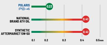
ASTM D4172. In 3rd party testing against 9 competitive products Polaris had 40% or better wear protection compared to all of the tested products. Numbers represent mm of wear scarring measured. Test measures wear at contact points, wear scar is measured for its length and width (in units of mm). Lower wear numbers mean better wear protection and friction reduction.
