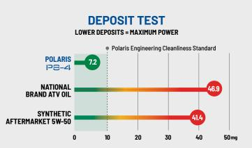
ASTM D6335. In 3rd party testing against 9 competitive products Polaris PS-4 had less than half the deposits compared to the next closest product. No other tested products met Polaris Engineering standards for deposit cleanliness. Test measure mass of deposits in mg in high temp, high stress test cycles. Higher deposits will impact engine power and performance.
