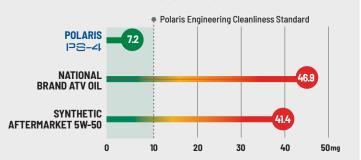
$ASTM\ D6335.\ In\ 3rd\ party\ testing\ against\ 9\ competitive\ products\ Polaris\ PS-4\ had\ less\ than\ half\ the\ deposits\ compared\ to$ the next closest product. No other tested products met Polaris Engineering standards for deposit cleanliness. Test measure mass of deposits in mg in high temp, high stress test cycles. Higher deposits will impact engine power and performance.
