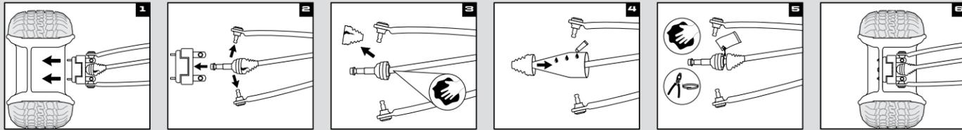
1. Remove wheel and axle nut.
